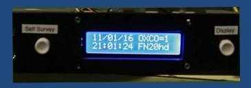
OCXO status, the definition is on page 5, under state machine. One of 8 possible states. 0 or 1 is normal operation when satellites are received. 0 time locked, 1 acquisition. 0 and 1 may toggle as satellites change.
