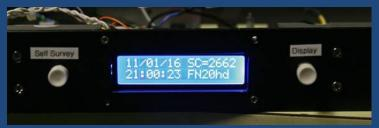
SC, Survey count, when self survey is being performed. Once self survey is done, this will be 0
